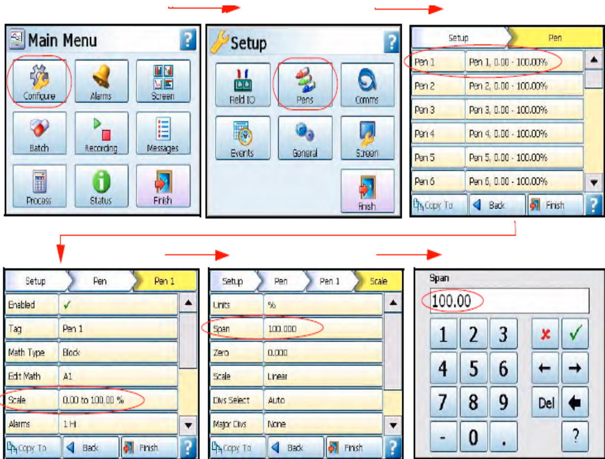
Example of a recorder menu path from the Main Menu to Pen Scale configuration with clear rapid navigation
